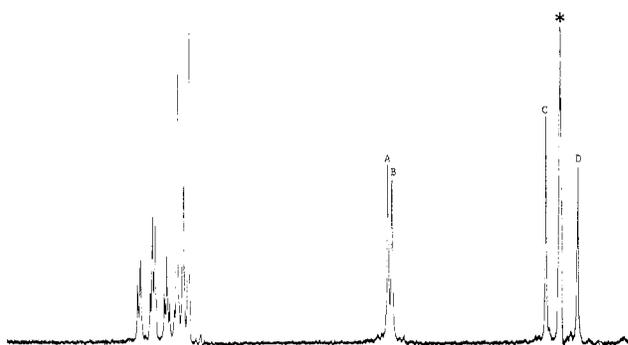
**Figure 4.** Low-temperature limiting  $^1\text{H}$  NMR spectrum of  $\text{W}_2(\text{NMe}_2)_4(\text{PhN}_3\text{Ph})_2$  ( $-45^\circ\text{C}$ ) 220 MHz in toluene- $d_8$ . Asterisk represents proton impurities in solvent.
